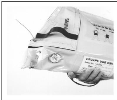
1. Check that the contents gauge needle is in the green sector, showing that the cylinder is fully-charged.
