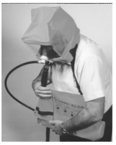
9. Check that there is a steady flow of air into the hood.
