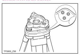
Level the instrument and then remove it from the tribrach. If the bubble is not centred, adjust it using the adjusting pin.
