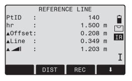
The calculated height difference is relative to the selected reference height (p | 1).
