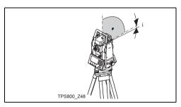
The vertical circle should read exactly 90° (100 gon) when the line of sight is horizontal. Any deviation from this figure is termed vertical index error (i). By determining the vertical index error the electronic level is adjusted automatically.
