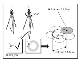
Depending on brightness and surface the size of the laser dot can vary. At a distance of 1.5 m an average value of 2.5 mm diameter must be estimated.
