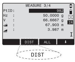
Under softkeys, a selection of commands and functions is listed at the bottom of the screen. They can be activated with the corresponding function keys. The available scope of each function depends on the applications / functions currently active.
