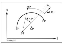
SP: Start point of arc EP: End point of arc
