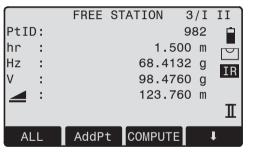
[ALL] Triggers angle and distance measurement (3 point resection).
