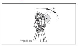
The line-of-sight error or collimation error (C) is the deviation from the perpendicular between the tilting axis and the line of sight.
