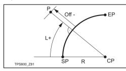
SP: Start point of arc EP: End point of arc
