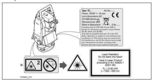
a) Will be replaced by a Class 3R warning label if applicable
