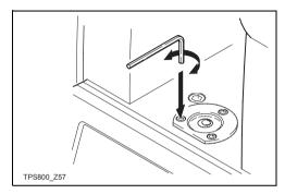
Level-up the instrument in advance with the electronic level. The bubble must be centered. If it extends beyond the circle, use the Allen key supplied to center it by turning the adjustment screws. After adjustment no screw must be loose.
