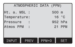
In order to take into consideration these influences distance measurements are corrected using atmospheric correction parameters.
