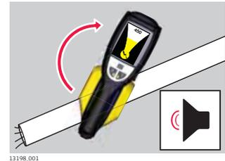
3. When the signal strength indicators are at a minimum, the blade of the locator is in line with the utility and indicates its direction.
