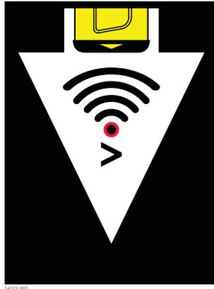
This screen indicates that the signal source is too high to provide a depth reading.
