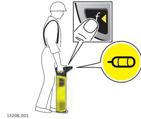
2. Position the locator directly over and in line with the sonde.
