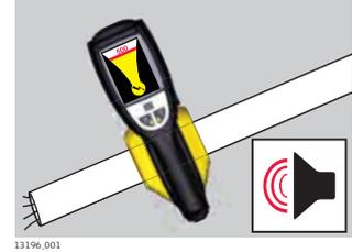
2. Rotate the Locator around its axis until the signal strength indicators are at a minimum.
