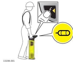
7. Walk in line with the suspected direction of travel observing the display. The signal strength indicator rises and falls as you pass over the ghost signal at the back of the sonde, the peak signal directly over the sonde and the ghost signal at the front. The Numeric Peak Indicator displays its highest value when detecting the peak signal.
