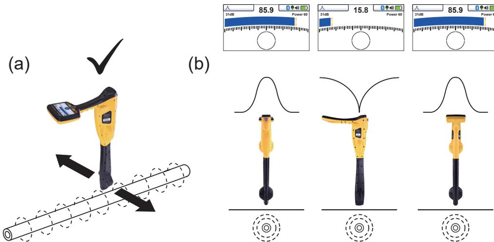
7. Rotate the vLoc3-Cam on its axis to obtain the maximum signal. The vLoc3-Cam is now directly over the line and with the blade across the line.
