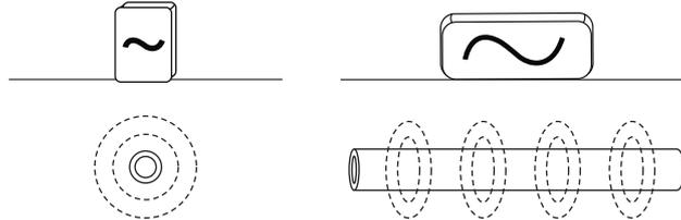
Remove any connections from the output connector. Switch on the transmitter and place it over the suspected position of the line and position it so that it is in line of the target as above. In the case of the Loc3-10Tx that is with the handle pointing along the line and in the case of other transmitters, arrows printed on the labels should point along the line of the target line.
