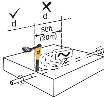
Also note that the signal will radiate out to the side of the transmitter as well as below. For this reason, it is recommended that when applying a signal using the induction method, a distance of at least 20m is kept from the transmitter when pinpointing or taking depth readings. Locating closer than 20m is possible but the operator should be aware that the signal directly received from the transmitter may be strong enough to influence the results.
