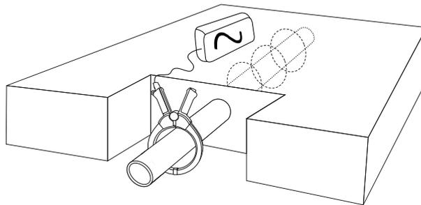
In many situations, it is not possible to gain access to a cable to make an electrical contact. Or if there is, it is not safe to do so. The signal clamp provides an efficient and safe method of applying a locate signal to a cable.
