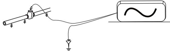
Active locating has the benefit that, unlike passive detecting, the operator is in control of the signals and therefore can be more specific about what line is detected. That is to say active signals can be used for line tracing. Also, passive signals are not always present on a line so using active signals ensures more lines are detected. (For passive locating see section 3.9)
