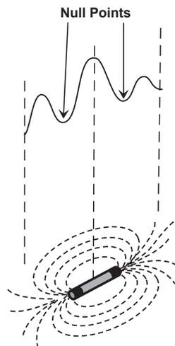
Due to this construction, the sonde gives a different “Peak” pattern note that there are three distinct peaks – a small peak – a large peak – a small peak with two “Nulls” between the peaks. The sonde is located under the center of the “large peak”.
