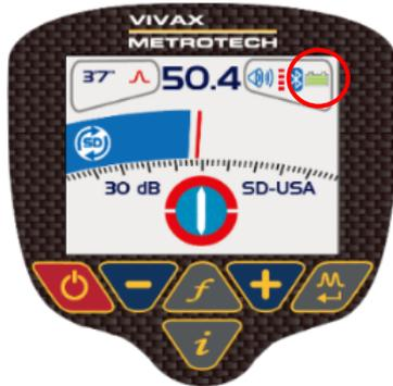
**vLoc2-- One to four red dots displayed near the Bluetooth icon**
