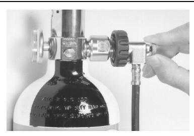
7. Close the compressor supply valve, bleed off pressure from the supply hose, disconnect the charging adaptor from the cylinder and fit the charging adaptor dust cover.
