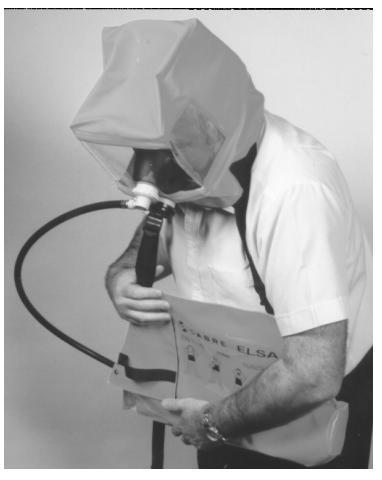
9. Check that there is a steady flow of air into the hood.
