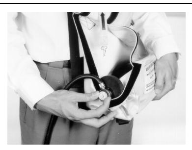
5. If there is still no sound, access the reducer/cylinder valve and pull the red EMERGENCY PULL disc.
