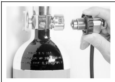
3. Fit 200 bar G5/8 pattern charging connector to the charging adaptor.
