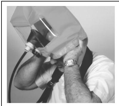
8. Hold the hood with the neck seal over the crown of the head and pull the hood down over the head until the neck seal is around the neck. Check that clothing or hair is not trapped in the neck seal.
